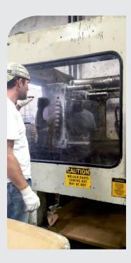
A machine operator waits for the custom injection molding machine to finish before releasing the cooler.
